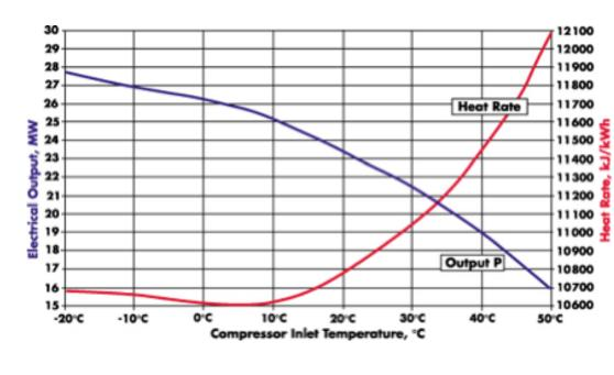
Generator output and heat rate versus compressor inlet air temperature for an SGT-600 industrial gas turbine (Siemens Westinghouse).
