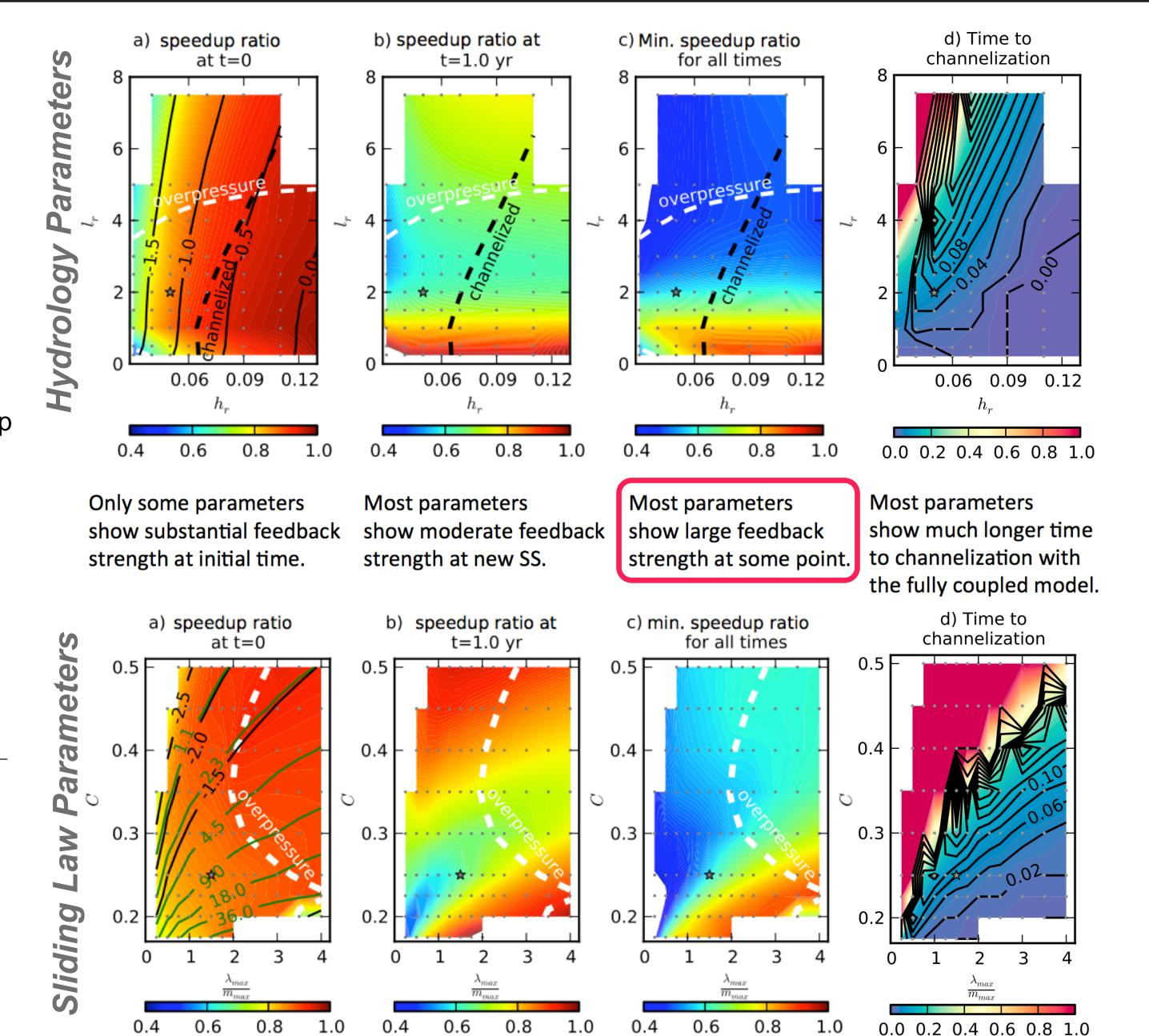
Black lines are contours of the log of meltwater input (m<sup>3</sup> s<sup>-1</sup>) required to achieve 4.55x speedup
