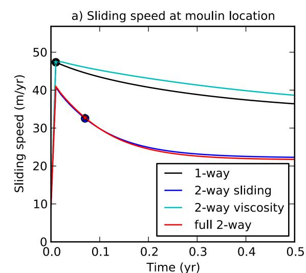
1-way: Hydrologic system adjusts to new input but slowly: new steady state water pressure and sliding velocity are lower than transient. 2-way velocity: Increased sliding opens subglacial cavities, lowering water pressure and sliding. (negative feedback)
