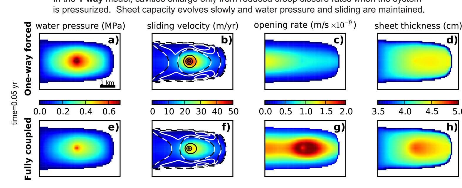
In the fully coupled model, sliding leads to increased cavity opening and a much larger capacity sheet. The increase in cavity size rapidly lowers water pressure and reduces sliding.
