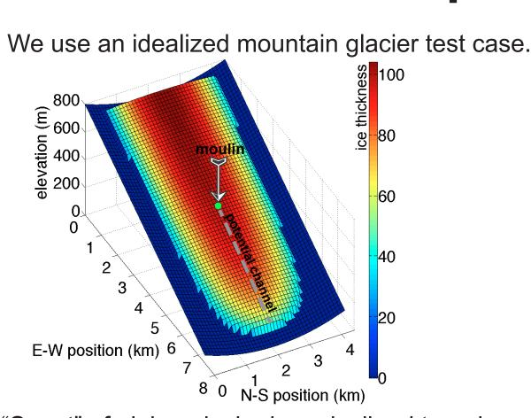
"Snout" of alpine glacier in an inclined trough: "Plastic glacier" shape (T<sub>c</sub>=10<sup>5</sup> Pa) 7 km long, 3 km wide
